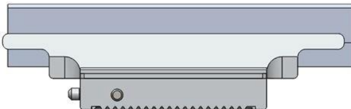
FIGURE 15. 11.5-INCH LONG PART PUSHED INTO PLACE USING Y PUSH TOOL
